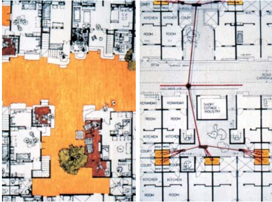
❖ Fig.4 Aranya-Acluster with 1 manhole for 18 service cores
