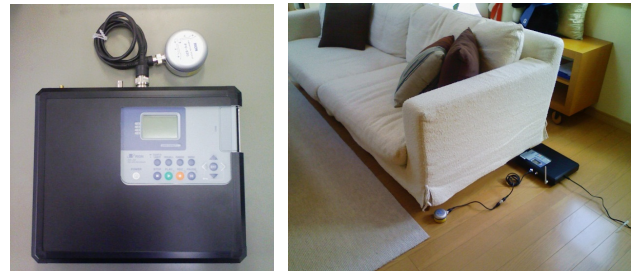
Fig. 1. Wireless vibration measurement device. Accelerometer dimensions: 67 (diameter) × 40.7 (height) mm; Weight: 370 g. Main unit dimensions: 50 (height) × 350 (width) × 250 (depth) mm; Weight: 2 kg.
