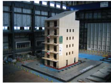
X-Lam shaking table test 2006,2007 CNR-IVALSA (Italy)
