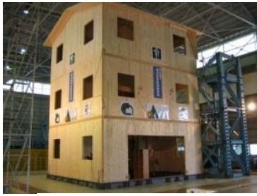
X-Lam shaking table test 2006,2007 CNR-IVALSA (Italy)
