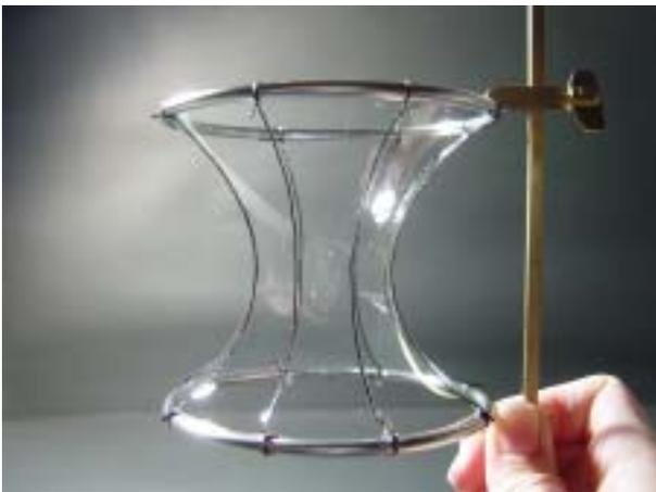
写真4、Catenoid Membrane with Cables-2
