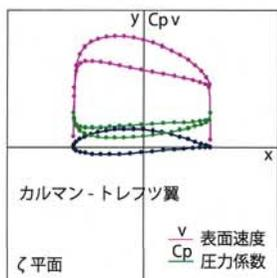
$$f(z) = U(z-z_0)e^{-i\theta} + \frac{Ua^2}{(z-z_0)e^{-i\theta}} + i\frac{\Gamma}{2\pi} \log(z-z_0)e^{-i\theta}$$
