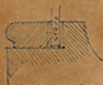
Single Glazing Basic Details for Stone openings, Loose Strips.
