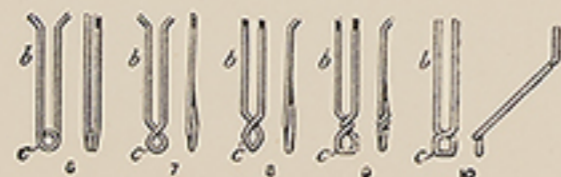
Fig. 5. Paragon System, Bracings.
